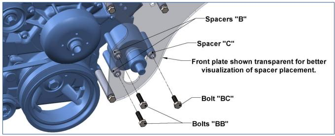
11. Install power steering pump bolts as shown (confirm P/S pump rear bracket was previously removed):
