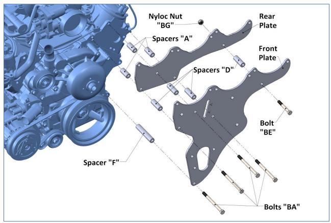
Apply supplied thread locker. Torque M10 bolts to 36 ft./lbs.
